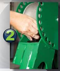
Position the Elbow to desired angle
