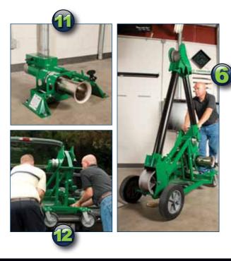
IMPROVED DESIGN! Interchangeable nose and elbow allows boom to be simply shortened for use in tight work spaces.
