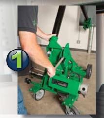
Lift the boom to desired angle using crank
