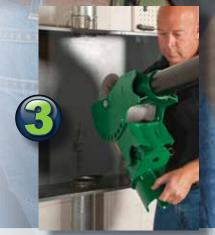
Position the Nose just over conduit and lower adapter into conduit by cranking the boom lower
