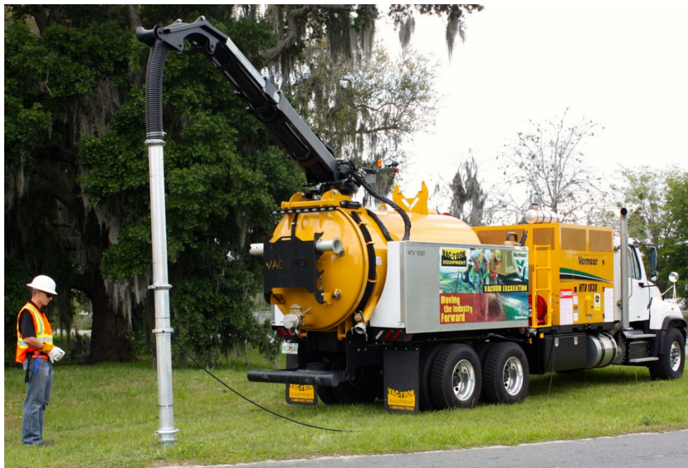
Figure 10.3: Typical Vacuum Pump Truck (courtesy of Vac-Tron Equipment, Inc.)
