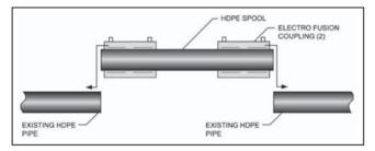
Figure 16 Electrofusion Repair Spool
