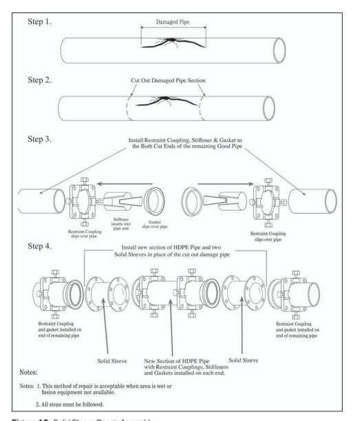
Figure 12 Solid Sleeve Repair Assembly
