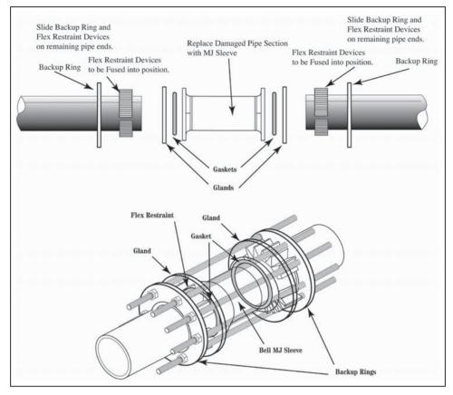
Figure 20 Mechanical Repair Fitting Restraint
