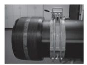
Figure 14 Hydraulic Re-Rounding Clamp Installed
