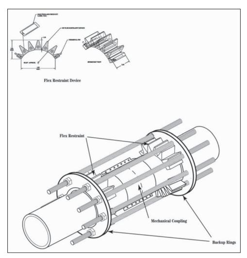
Figure 21 Mechanical Coupling Restraint
