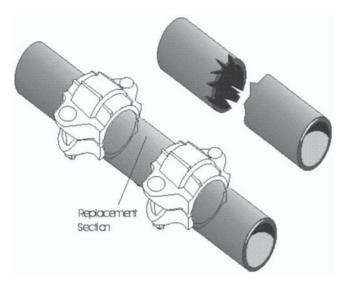
Figure 10 Mechanical Coupling Repair Assembly
