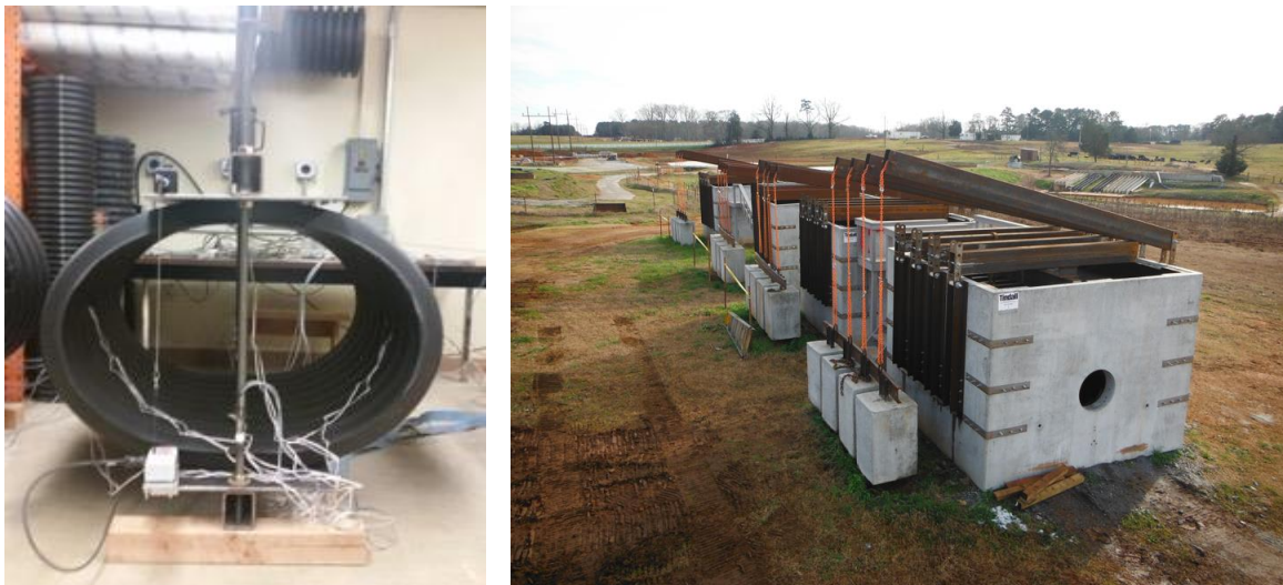
Figure 8.9: Laboratory and field testing on full scale pipes to validate the service life prediction model established by shifting elevated temperature UCLS data to service conditions.
